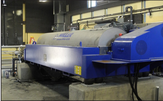
Centrifuge for mechanical dewatering of sludge
